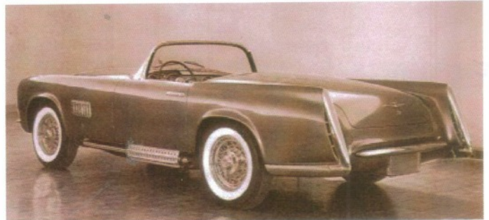
Three Falcon concept cars were built by Chrysler's Advanced Styling Studio, each with a 105-inch wheelbase and 170-horsepower DeSoto Hemi V-8.
