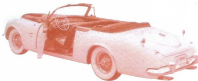
The C-200 was built on a production Chrysler Saratoga chassis and featured "gunsight" taillamps.
